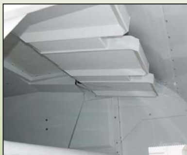
Unique roof-mounted paddle packer minimizes CA and generates 73,000 lbs packing force.
