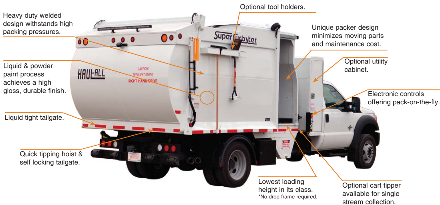
Unique roof-mounted paddle packer minimizes CA and generates 73,000 lbs packing force.
