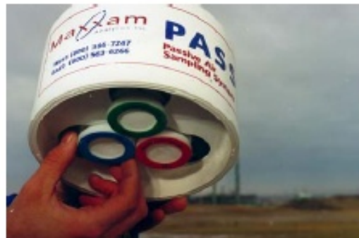
Figure F-3 Removal and disassembly of the passive sampler after exposure
