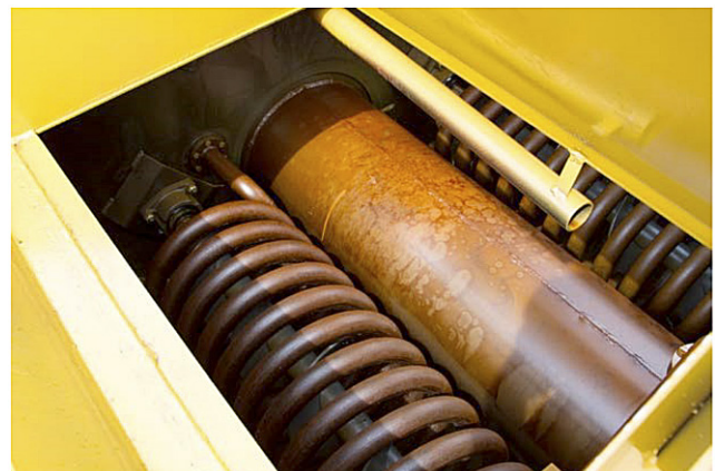
Figure 6 Circulating Augers Inside Heat Coiling
