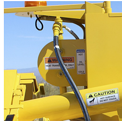
Figure 10 Hot-Oil Expansion Tank
