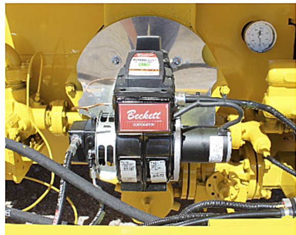
Figure 9 Diesel Fuel Burner
