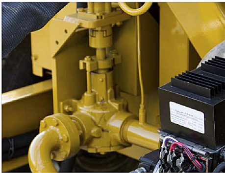
Figure 7 Heat-Transfer Oil Pump
