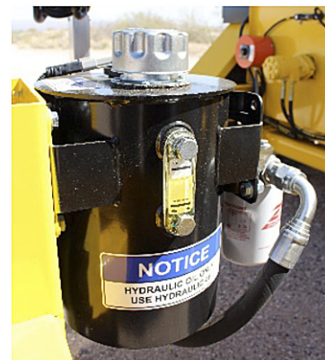
Figure 3. Hydraulic Reservoir & Filter
