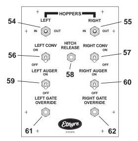
Figure 9. Front Operator's Control Panel
