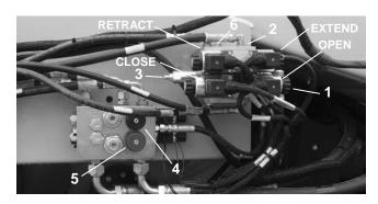
Figure 33. Left Hopper Valves
