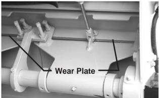
Figure 14. Hopper Gate Wear Plate
