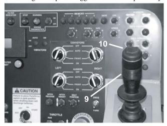
Figure 5. Speed/Direction Control Handle
