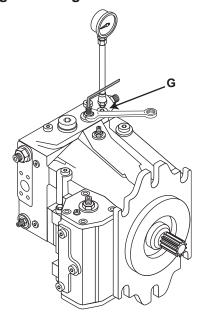
Figure 26. Charge Pressure Adjustment
