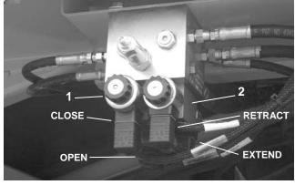
Figure 21. Right Gate Solenoid
