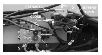
Figure 30. Left Hopper Valves
