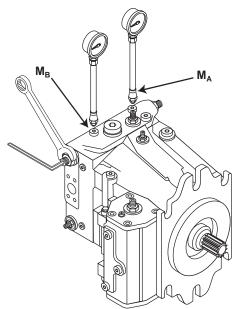
Figure 25. High Pressure Relief Setting
