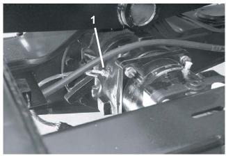
Figure 6. Ground Speed Pickup
