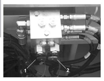
Figure 29. Right Auger/ Spread Roll Manifold
