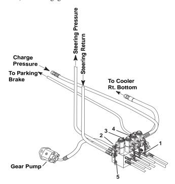
Figure 35. Hydraulic Control Assembly
