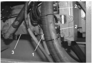
Figure 17. Hydrostatic Pump
