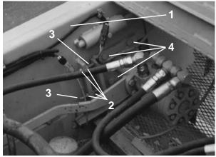
Figure 16. Conveyor Head Pulley Adjustment
