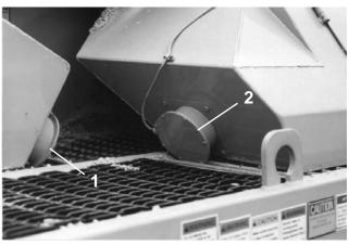
Figure 10. Conveyor Diaphragm Switches
