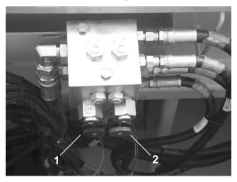
Figure 32. Right Auger/Spreadroll Manifold
