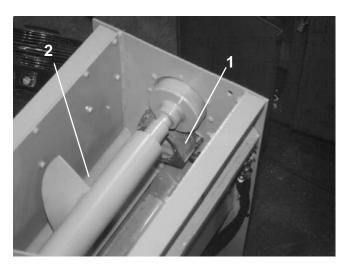
Figure 8. Auger Auto On/Off Switch
