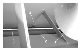
Figure 13. Spread Roll Wear Plate
