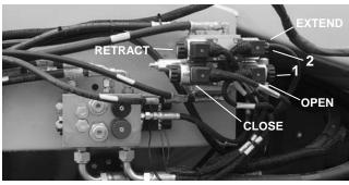
Figure 20. Left Gate Solenoid
