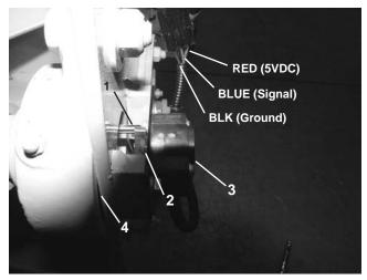
Figure 22. Left Hopper Transducer
